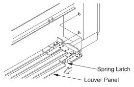
Figure 36 - Removing Louver Panel
